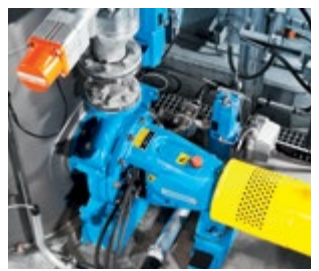
PM2's new generation MC pump with patented SMARTSEP technology.
