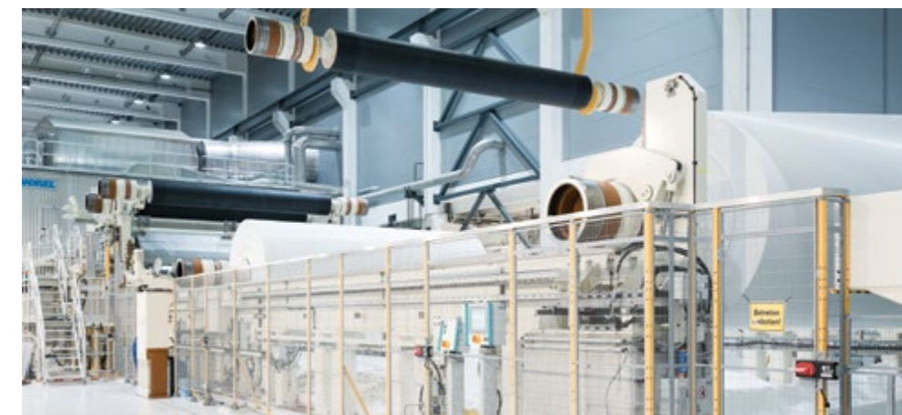
Fully automated tambour change that minimizes maintenance.
